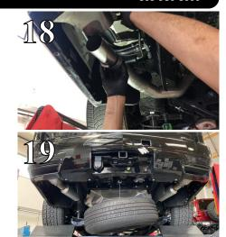
WARNING: Use extreme caution during installation. Torque all fasteners according to manufacturer's torque values and tightening sequence. <u>DO NOT</u> use air impact tools to tighten fasteners on Borla Performance Exhaust Systems. Use of such tools may result in bent flanges or gasket contact areas leading to exhaust leaks.
