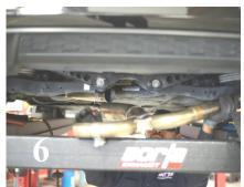
WARNING: Use extreme caution during installation. Torque all fasteners according to manufacturer's torque values and tightening sequence. <u>DO NOT</u> use air impact tools to tighten fasteners on Borla Performance Exhaust Systems. Use of such tools may result in bent flanges or gasket contact areas leading to exhaust leaks.
