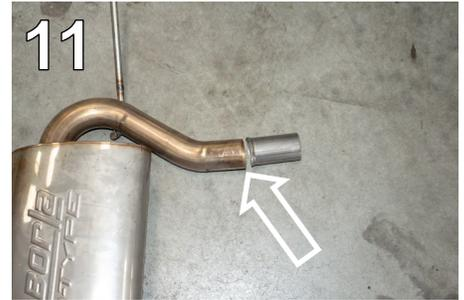
1. Make a cut on the inlet pipe of your Axle-Back exhaust (PN 11961) as shown (fig. 11).
