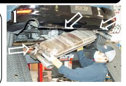
Note: With a used vehicle, we suggest a penetrating spray lubricant to be applied liberally to all exhaust fasteners and allowing a significant period of time for the chemical to lubricate the threads before attempting to disassemble.
