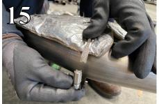
WARNING: Use extreme caution during installation. Torque all fasteners according to manufacturer's torque values and tightening sequence. <u>DO NOT</u> use air impact tools to tighten fasteners on Borla Performance Exhaust Systems. Use of such tools may result in bent flanges or gasket contact areas leading to exhaust leaks.
