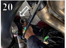
WARNING: Use extreme caution during installation. Torque all fasteners according to manufacturer's torque values and tightening sequence. <u>DO NOT</u> use air impact tools to tighten fasteners on Borla Performance Exhaust Systems. Use of such tools may result in bent flanges or gasket contact areas leading to exhaust leaks.
