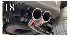
WARNING: Use extreme caution during installation. Torque all fasteners according to manufacturer's torque values and tightening sequence. <u>DO NOT</u> use air impact tools to tighten fasteners on Borla Performance Exhaust Systems. Use of such tools may result in bent flanges or gasket contact areas leading to exhaust leaks.
